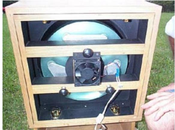
**Above is Lee Troske's 8 inch scope. He designed his scope so that the primary mirror and mirror cell are easy to remove. The four latches make this possible. A fan is used to cool the primary mirror for the night time viewing to come.**
