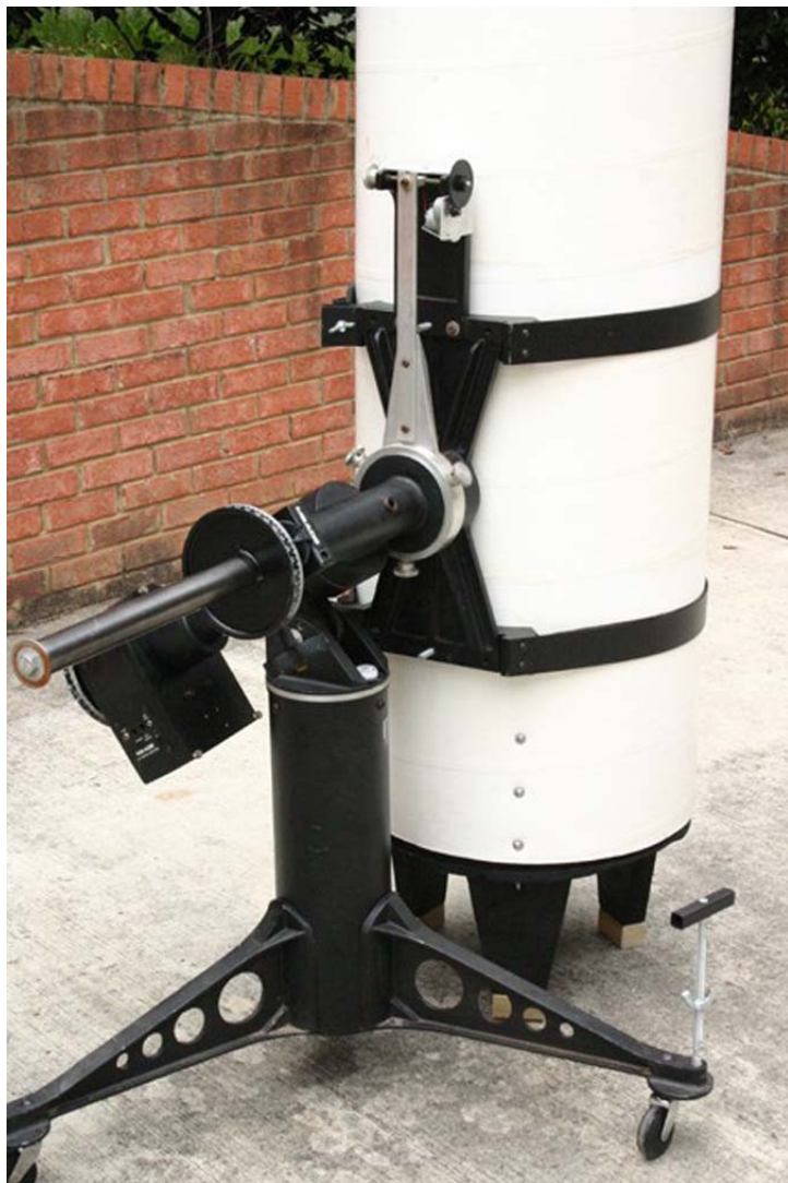
The use of the “OTA stool” is shown here (attached under the OTA). One simply sets the OTA upright on the ground at the setup site. It’s then a simple matter of rolling the mount to the scope and sliding the mounting bolts through the holes to complete the attachment.
