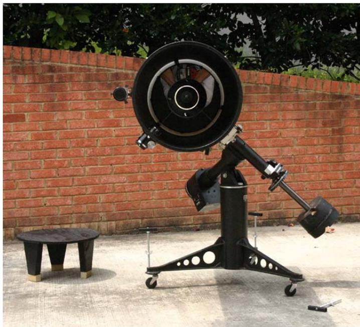
*This is a view down the business end of the big scope after replacing the mounting stool with the primary mirror cell.*
