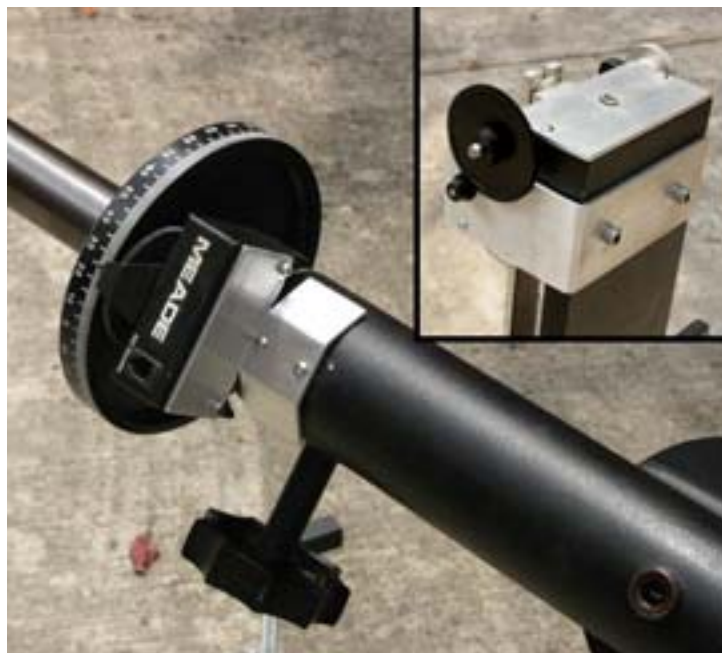
This is a view of the newly fabricated DEC encoder bracket (left – polished aluminum) and DEC slow motion assembly (upper right – polished aluminum parts). The original encoder bracket used only one screw and was a mere ½” wide causing the encoder to frequently bend away from the DEC shaft gear. The original slow motion assembly was equally fragile and would become misaligned with the slightest touch.
