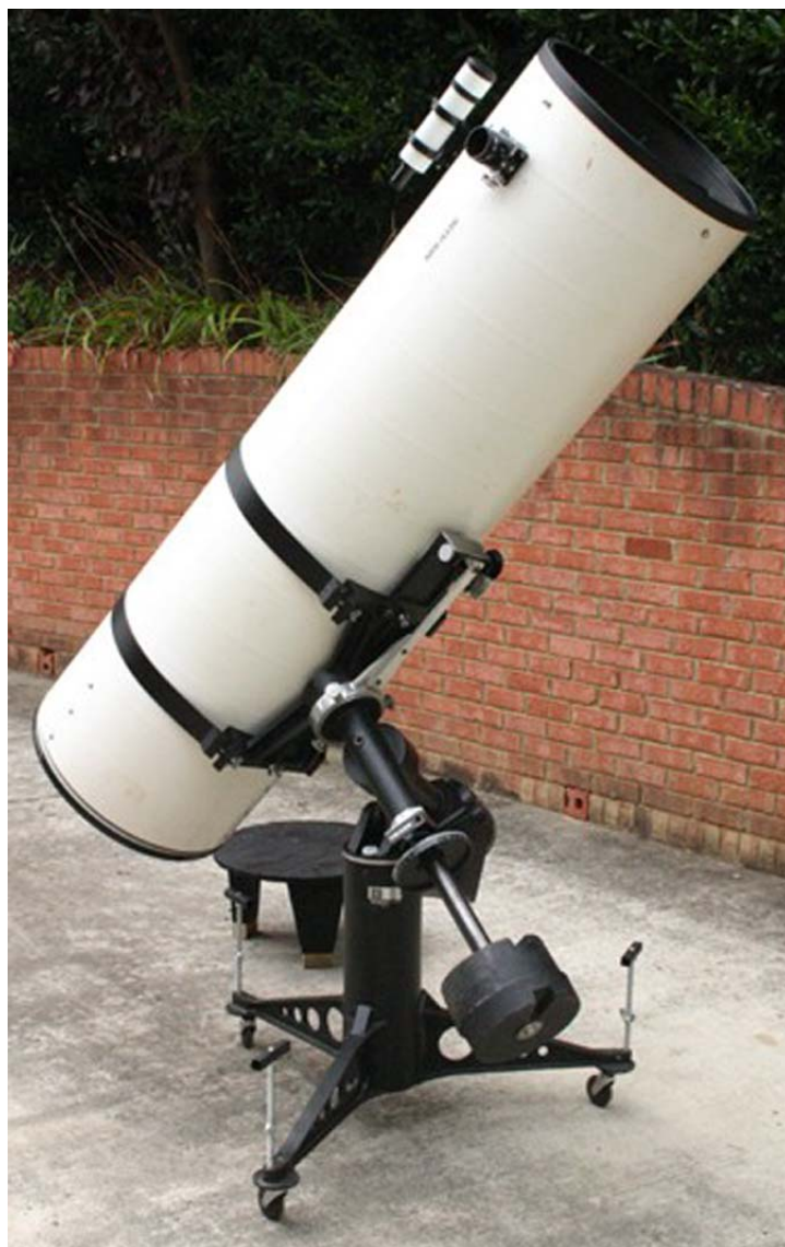
The fully assembled Starfinder 16 is shown here, ready to be rolled over to a set of polar alignment marks on the concrete where it can be easily leveled and secured with the leg jacks.
