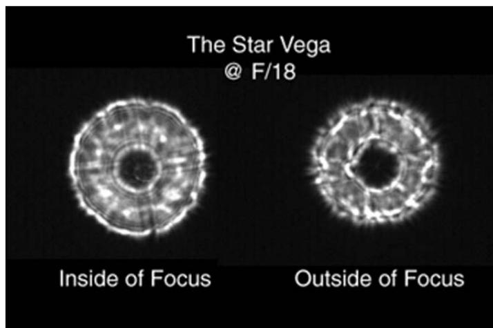
The diffraction patterns of stars, photographed inside and outside of focus at high power provide clues to the optical quality of a telescope. In this star test of the Starfinder’s optics, notice that the “inside” pattern exhibits a bright ring around the outer edge. The “outside” image has no bright ring. This indicates that the optics are a bit “undercorrected”. In other words, the curve of the mirror is somewhere between a sphere and the ideal shape of a parabola.
