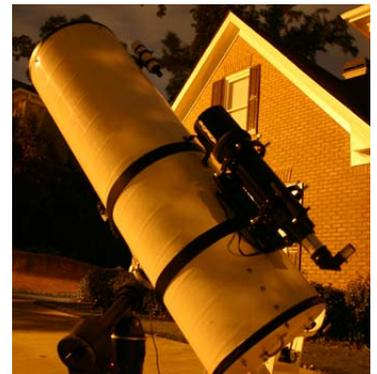
*This is a view of the Starfinder with a 5" refractor attached. The refractor proved to be essential for finding deep sky objects when not using the Magellan II computer. A dovetail adapter was added so that standard Losmandy attachments could be used.*
