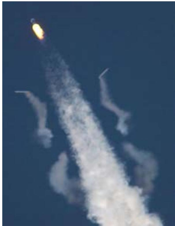
*This image shows the Solid Rocket Boosters separating from the Delta II rocket.
