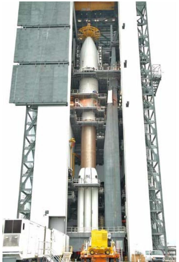
*The New Horizons launch vehicle fully assembled at Cape Canaveral Launch Complex 41. Credit NASA/JHU/APL*
