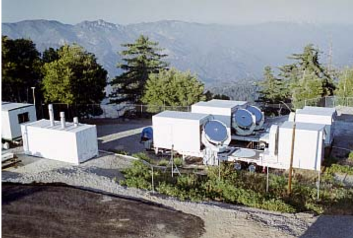
The three telescopes of the Infrared Spatial Interferometer lined up east-west on Mt. Wilson in Southern California. The telescopes are mounted in semi-trailers so that they can be moved. The building with the periscopes houses a laser which is transmitted to all three telescopes (David Hale 2006)
