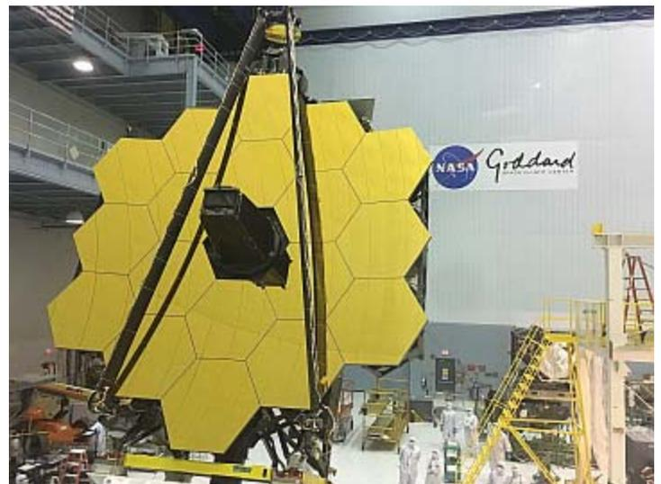
The JWST optical assembly after its completion in the clean room at NASA Goddard last year. The optical assembly was then integrated with the Science Instrument Module. This assembly will then be shipped to Northrup Grumman to be integrated with the Spacecraft Bus, which will provide electrical power, communications, computing, propulsion, and thermal control. NASA image.
